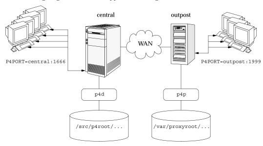
In this configuration, file revisions requested by users at a remote development site are fetched first from a central Perforce server (p4d running on central) and transferred over a relatively slow WAN. Subsequent requests for that same revision, however, are delivered from the Perforce Proxy, (p4p running on outpost), over the remote development site's LAN, reducing both network traffic across the WAN and CPU load on the central server.
