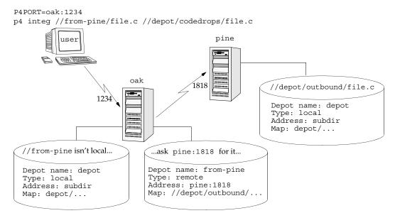
Although it is possible to permit individual developers to sync files from remote depots into their client workspaces, this is generally an inefficient use of resources.
