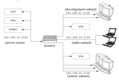
Deploying an additional proxy server on a subnet when network bandwidth on the subnet is nearly saturated will not likely result in a performance improvement. Instead, split the subnet into multiple subnets and deploy a proxy server in each resulting subnet.
