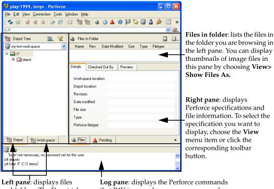
**Left pane**: displays files and folders. The Depot tab displays files in the Perforce server, and the Workspace tab displays files in the workspace on your computer **Log pane**: displays the Perforce commands that P4V issues, plus error messages and results.
