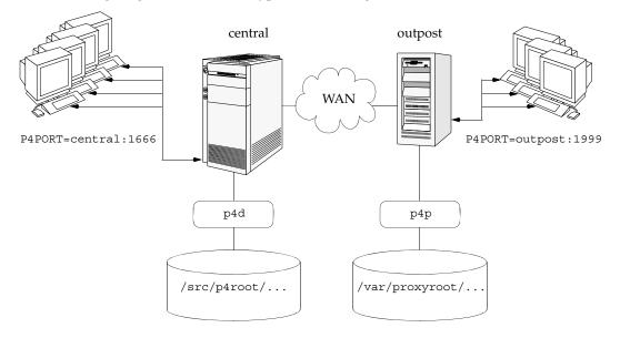
The following diagram illustrates a typical P4P configuration.
