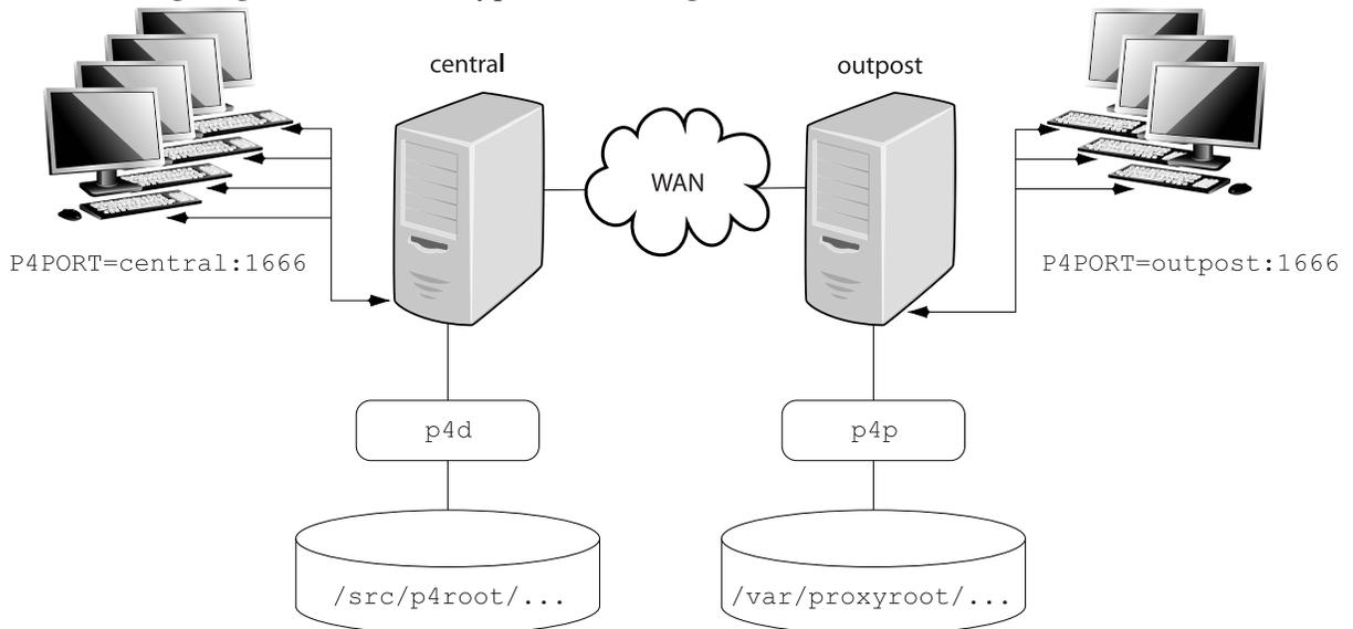
In this configuration, file revisions requested by users at a remote development site are fetched first from a central Perforce server (**p4d** running on **central**) and transferred over a relatively slow WAN. Subsequent requests for that same revision, however, are delivered from the Perforce Proxy, (**p4p** running on **outpost**), over the remote development site's LAN, reducing both network traffic across the WAN and CPU load on the central server.
