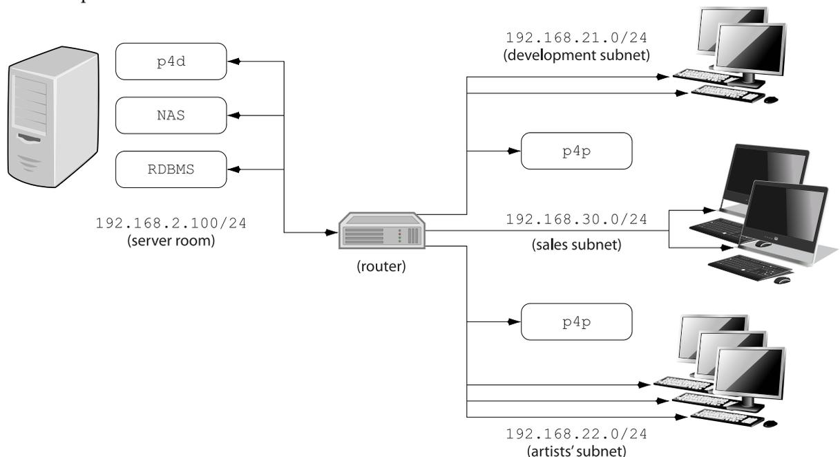
Deploying an additional proxy on a subnet when network bandwidth on the subnet is nearly saturated will not likely result in a performance improvement. Instead, split the subnet into multiple subnets and deploy a proxy in each resulting subnet.
