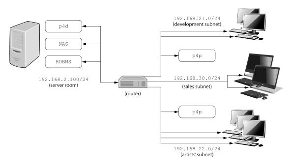
Deploying an additional proxy on a subnet when network bandwidth on the subnet is nearly saturated will not likely result in a performance improvement. Instead, split the subnet into multiple subnets and deploy a proxy in each resulting subnet.
