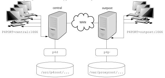
The following diagram illustrates a typical P4P configuration.
