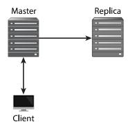
When you create the replica, you specify which server it should get its data from. The replica then periodically updates itself by copying files and metadata from the master. If the master fails, all you need do is reconfigure the replica to be the new master and then reconnect clients to communicate with it.
