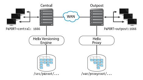
The following diagram illustrates a typical proxy configuration:
