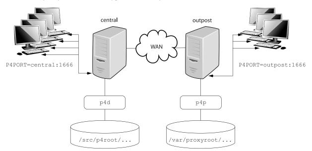
The following diagram illustrates a typical P4P configuration.
