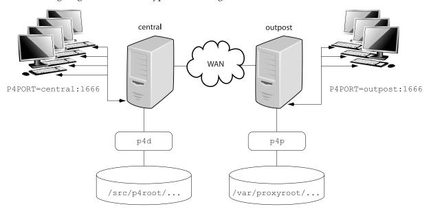
In this configuration, file revisions requested by users at a remote development site are fetched first from a central Perforce server (p4d running on central) and transferred over a relatively slow WAN. Subsequent requests for that same revision, however, are delivered from the Perforce Proxy, (p4p running on outpost), over the remote development site's LAN, reducing both network traffic across the WAN and CPU load on the central server.
